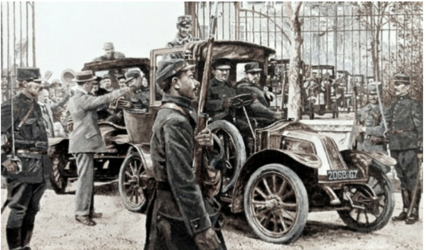
The taxis of 1914 were Renault AG1 Landaulets seating five men and averaging about 20-25 miles per hour – Public domain, guerre 14-18.org
