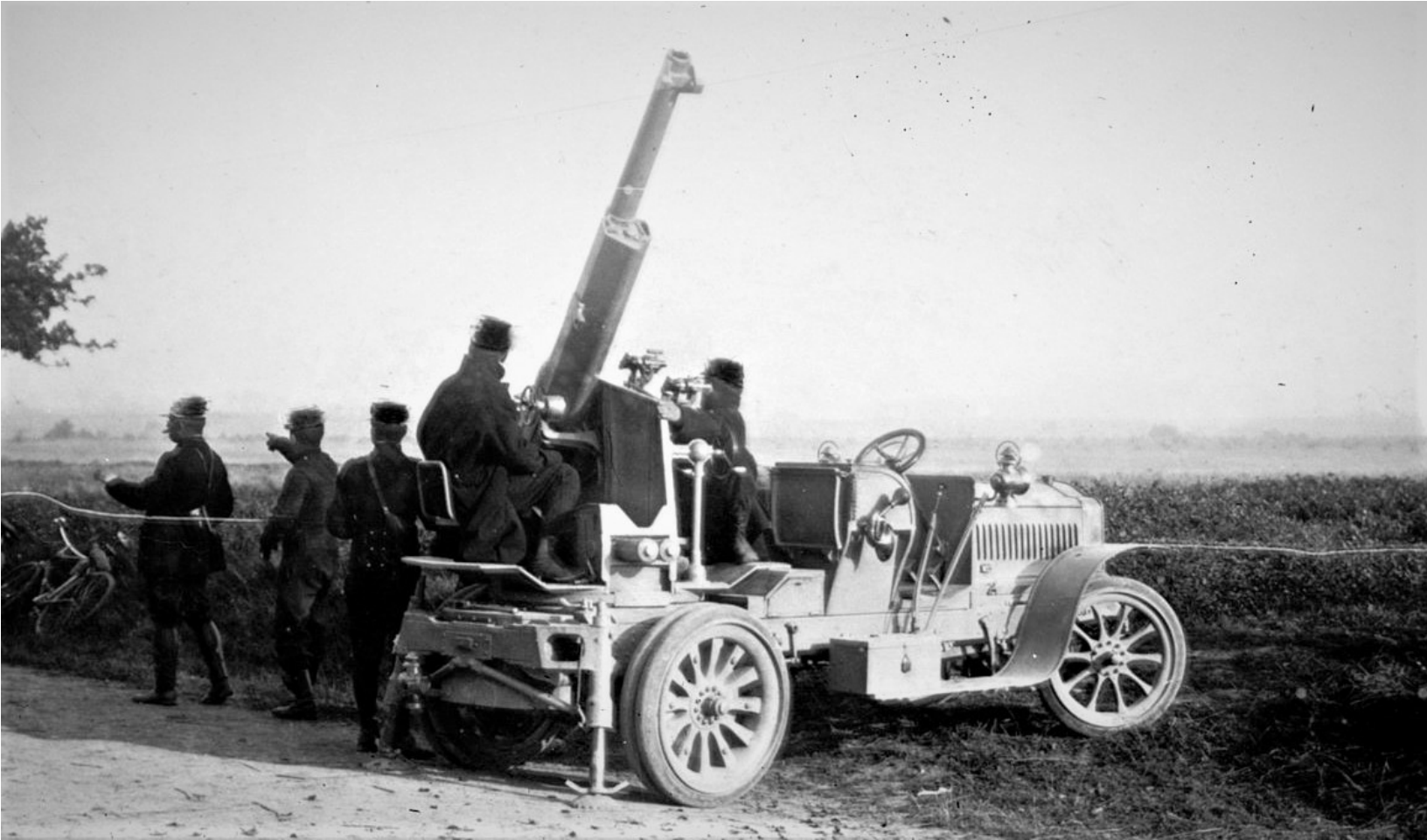
Self-propelled anti-aircraft mounting of the French 75 gun defending Paris – Unknown author, public domain. U.S. Library of Congress, Wikimedia
